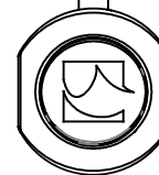
Detail 1:1 bottom rail Slim 25 cable guided
